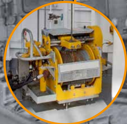
1. Tugger Load Monitoring optimizes general lifting operations on the drill floor
