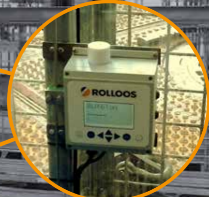
3. Lifted load constantly indicated on safe area and Ex displays
